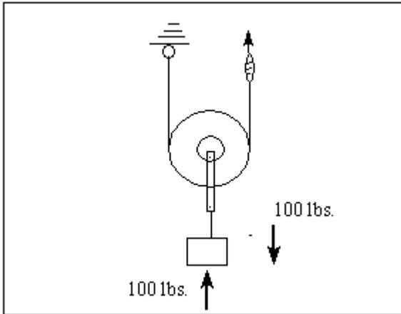
In many applications, both fixed and moveable pulleys are used in combination to form a device known as a **block and tackle**. A block and tackle is capable of both changing the direction of a force and creating a mechanical advantage.
