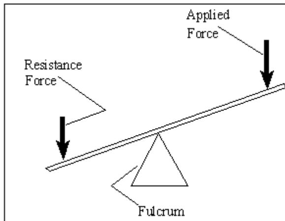
The mechanical advantage of a lever is the ratio of the length of the lever on the applied force side of the fulcrum to the length of the lever on the resistance force side of the fulcrum. The mechanical advantage of the lever below is 10:1. Therefore, an applied force of 10 pounds will balance a resistance force of 100 pounds. However, the applied force end of the lever must move 10 feet for every one foot the resistance force is raised.
