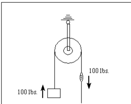
A pulley is said to be a fixed pulley if it does not rise or fall with the load being moved. A fixed pulley changes the direction of a force; however, it does not create a mechanical advantage. A fixed pulley is illustrated below.
